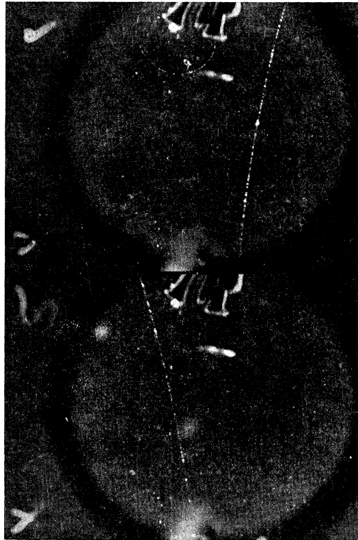
FIG. 6. A positive and a negative meson track photographed on adjacent frames of the same film strip (carbon specimen). The sharply curved negative track at the top of the upper picture is known not to be contemporaneous with the meson track since its narrow width indicates that that particle passed through the cloud chamber after the expansion.
