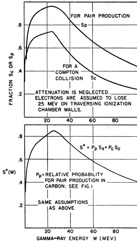
FIG. 2. Above: Fraction of gamma-ray energy which goes into ionization after one collision. Below: Average fraction of gamma-ray energy which goes into ionization after one collision in carbon. (The equation between the abscissae .6 and .8 should read:  $S^0 = P_p S_p + P_c S_c$ .)
