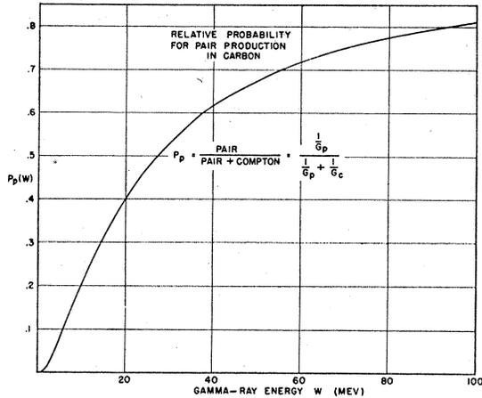
FIG. 1b. Relative probability for pair production in carbon.
