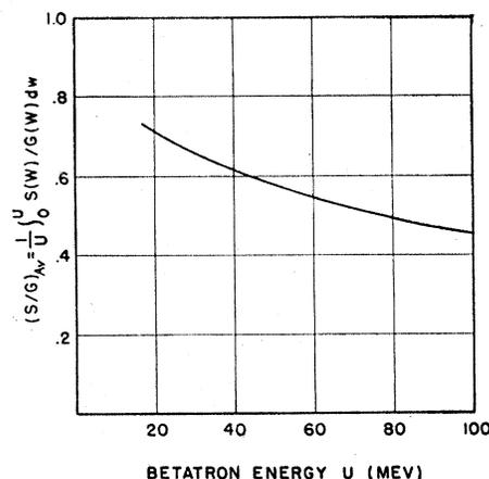
FIG. 4. Fraction of incident gamma-ray energy converted to ionization per radiation length if incident intensity is flat from 0 to  $U$  Mev. Ionization energy in gas layer = (incident energy)  $\langle S/G \rangle_{Av} \Delta t (R_c/R_g)$ , where  $\Delta t$  is the thickness of gas layer in radiation lengths, and  $R_c/R_g$  is the ratio of electron ranges in carbon and in the gas, both measured in radiation lengths.
