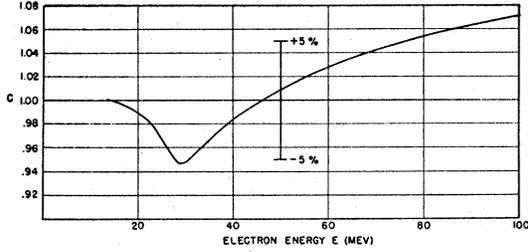
FIG. 5.  $C$  is the ratio of the actual fraction of electron energy converted to ionization, to the fraction used for computation in this paper.  $C = \eta(\text{actual})/\eta(\text{used})$ . The fraction used was: for  $E < 25$  Mev,  $e^{-T/G}$ ; for  $E > 25$  Mev,  $(25/E)e^{-T/G}$ . The actual fraction takes into account attenuation, radiation, scattering and non-linear range-energy relationship.
