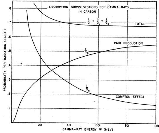
FIG. 1a. Absorption cross sections for gamma-rays in carbon.
