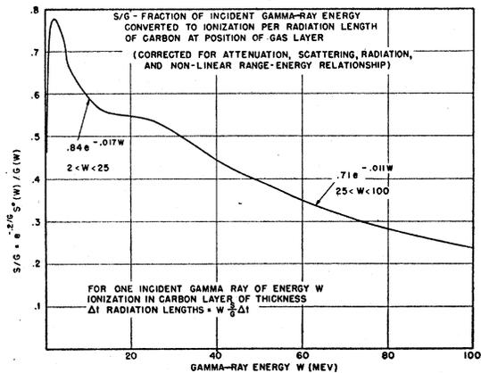
FIG. 3.  $S/G$  is fraction of incident gamma-ray energy converted to ionization per radiation length of carbon at position of gas layer (corrected for attenuation, scattering, radiation, and non-linear range-energy relationships).
