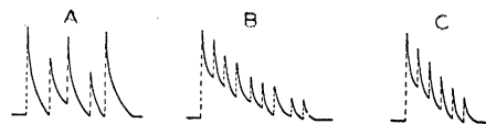
FIG. 2. A: Irregular Trichel-pulse burst in dry, clean air near onset of negative corona (7000 volts). B: The same in 6 percent freon in air, p=745 mm of Hg. C: The same in 10 percent freon in air, p=745 mm of Hg. It is possible that the individual pulses in B and C return to the zero line. Because of the high speed of pulse formation (less than one microsecond) the details of this oscillograph trace must be instrumental, but the general decay of the pulses seems to be real.
