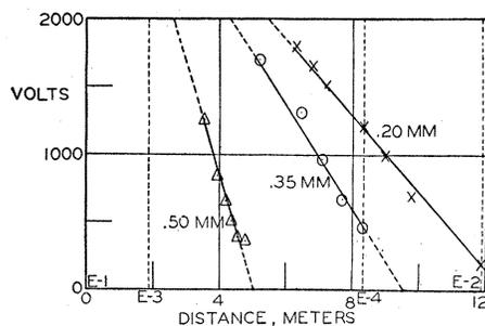
FIG. 7. Maximum positive potential above ground as function of distance with  $E-3$  grounded and conditions same as for Fig. 6.
