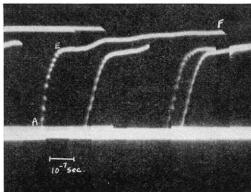
FIG. 4. Several oscillograms of potential from *E-4* to ground. The maximum of the initial rise is at *E* and the final maximum at *F*. Hydrogen at 2.5 mm Hg pressure, -85 kv applied potential.
