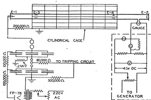
FIG. 1. Diagram of discharge tube with Marx circuit, cylindrical shielding cage, vacuum gauge circuit, and electrodes. Distance from E-3 to E-4 is 642 cm. Resistance values are approximate.
