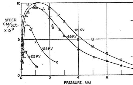
FIG. 3. Speed-pressure curves for high potential discharge in air. Negative applied potential.
