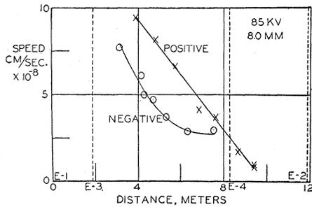
FIG. 5. Speed-distance curves of low potential discharge in air at 8.0 mm pressure and with 85 kv applied potential. Position of fixed electrodes is indicated by vertical dotted lines.
