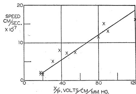
FIG. 8. Speed of low potential discharge in air as function of  $X/p$  for pressures of 0.20 mm to 0.50 mm Hg and for positive potential. Lowest speed  $1.7 \times 10^7$  cm/sec at  $X/p$  about 20.
