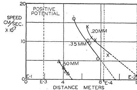
FIG. 6. Speed-distance curves of low potential discharge in air with E-3 grounded.
