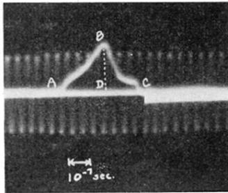
FIG. 2. Oscillogram for computing speed in air at 0.034 mm Hg pressure with  $-85$  kv applied potential. Frequency of timing wave is 19.0 megacycles per sec.
