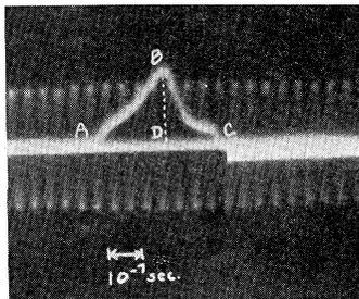
FIG. 2. Oscillogram for computing speed in air at 0.034 mm Hg pressure with  $-85$  kv applied potential. Frequency of timing wave is 19.0 megacycles per sec.
