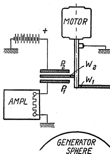
FIG. 1. Rotating compensation voltmeter.
