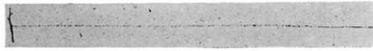
FIG. 2. Ternary fission: third fragment—mass \approx 6 , range=44 cm air equivalent. The two branches on one of the heavy fragments are caused by nuclear collisions.
