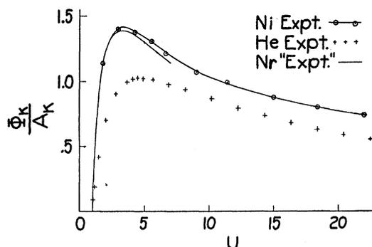
FIG. 5. Comparison of Smith's cross sections for He with those of Ni and the hypothetical non-relativistic element Nr, showing how something, presumably the electron which remains in the He atom, gives He abnormally small ionization cross sections at low  $U$ 's.
