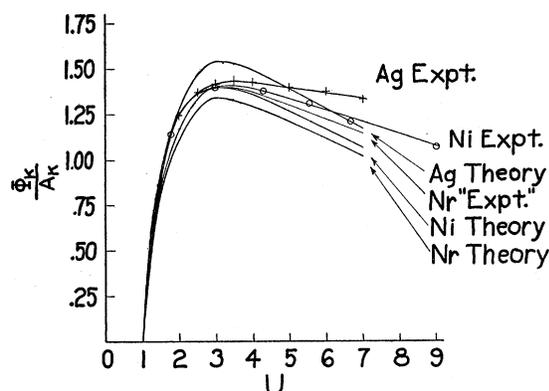
FIG. 4. Comparison of Ag with Ni, showing the effect of relativity; and graphs obtained by extrapolation for a hypothetical non-relativistic element Nr, showing how Burhop's non-relativistic theory fits this element best.
