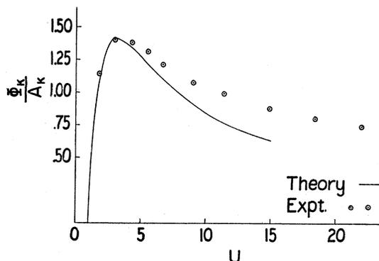
FIG. 3. Comparison of Burhop's theory with experimental cross sections for  $K$  ionization of nickel atoms.
