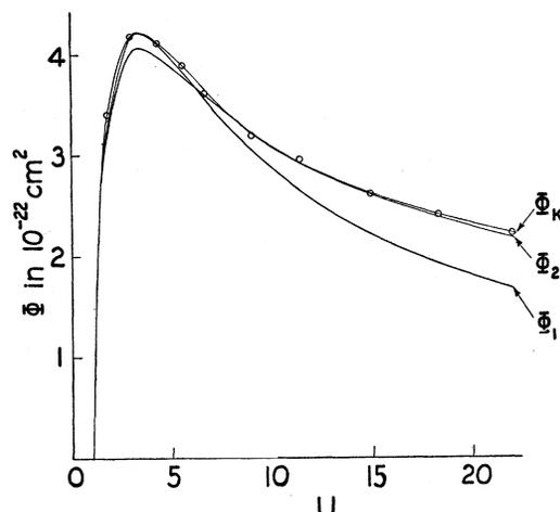
FIG. 2. Graph and points for experimentally determined  $K$ -ionization cross sections of nickel atoms (not single  $K$  electrons) and graphs of the empirical functions defined in Eqs. (2) and (3).
