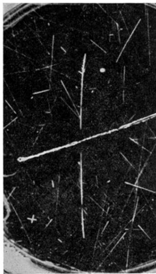
FIG. 4. Paired fragment tracks in hydrogen. The up-going fragment track appears with two long proton branches, one close after the other, both suitable for velocity determination.
