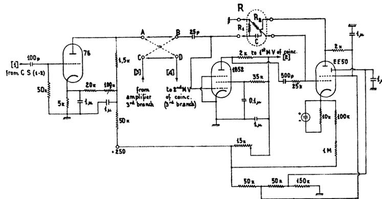
FIG. 5. First coincidence multivibrator.
