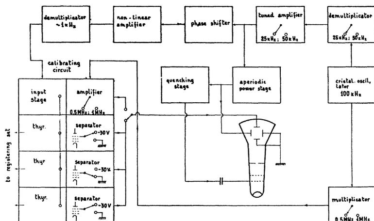
FIG. 9. Block diagram of calibrating set.
