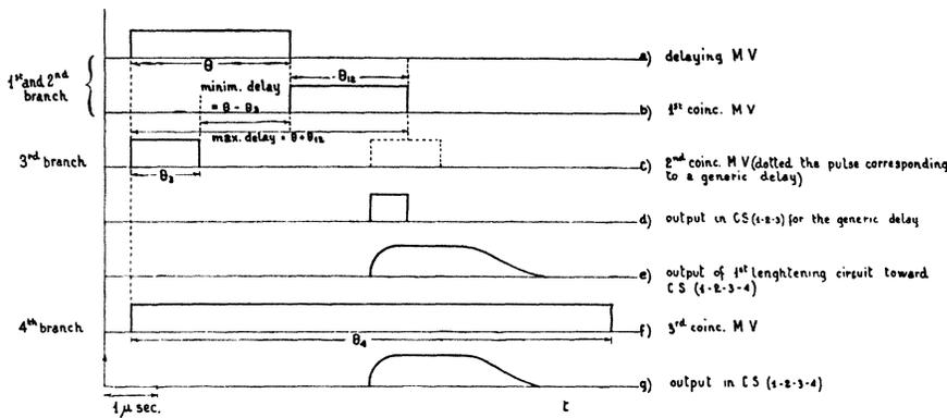
FIG. 7. Schematic diagram showing the time distribution of pulses.
