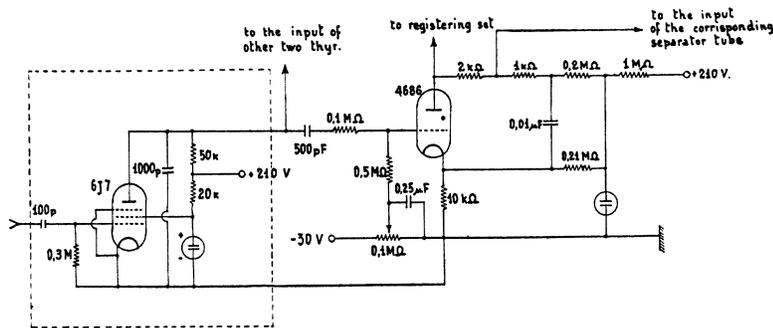
FIG. 11. Separator tube (three identical stages) and amplifier of the 0.5–1.0 MHz signal.
