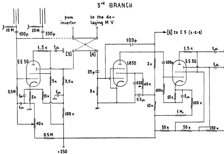
FIG. 6. Input amplifier (third branch) and second coincidence multivibrator.
