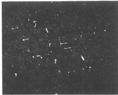
FIG. 15. Trigonal path set in basal quartz.
