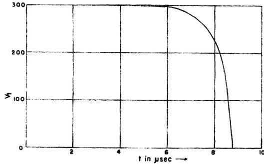
FIG. 5. Voltage across thyatron as a function of time as plotted from Eqs. (16) and (17) with  $V_a=10$  volts,  $E_b=300$  volts, and  $R_p=10,000$  ohms. The grid overvoltage is applied at  $t=0$ .
