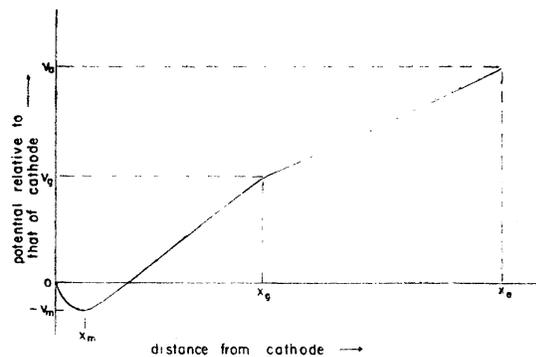
FIG. 3. Potential distribution (along a line joining cathode and anode and passing through a grid hole) across tube immediately after the application of a grid overvoltage,  $V_g$ .  $X_g$  and  $X_a$  are the distances of grid and anode from the cathode, respectively;  $V_a$  is the anode voltage. The potential minimum,  $-V_m$ , occurring at  $X_m$ , is caused by electron space charge.
