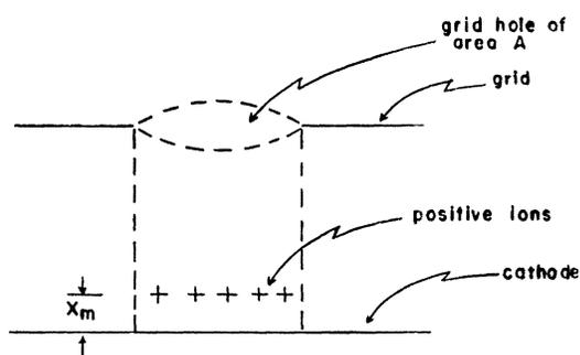
FIG. 4. The layer of positive ions and the cathode form a small parallel plate condenser of area  $A$  and thickness  $X_m$ .
