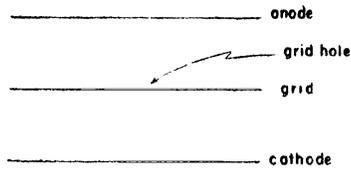
FIG. 2. Model of thyatron assumed for derivation of the equation describing the initiation of discharge. The anode, grid, and cathode are assumed to be parallel plane electrodes.
