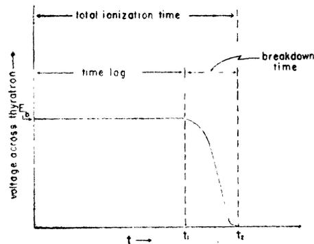
FIG. 1. Typical curve for voltage drop across thyatron as a function of time after application of grid overvoltage (at  $t=0$ ).  $E_b$  is the power supply voltage.
