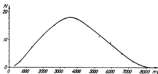
FIG. 1. The  $\beta$ -spectrum of  $I^{128}$ .
