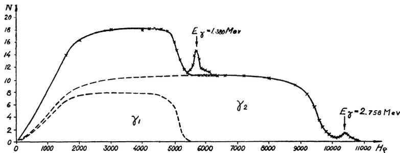
FIG. 3. Secondary electron spectrum expelled from a Cu radiator covered with a 0.02-mm Pb-foil by the  $\gamma$ -rays of  $\text{Na}^{24}$ .
