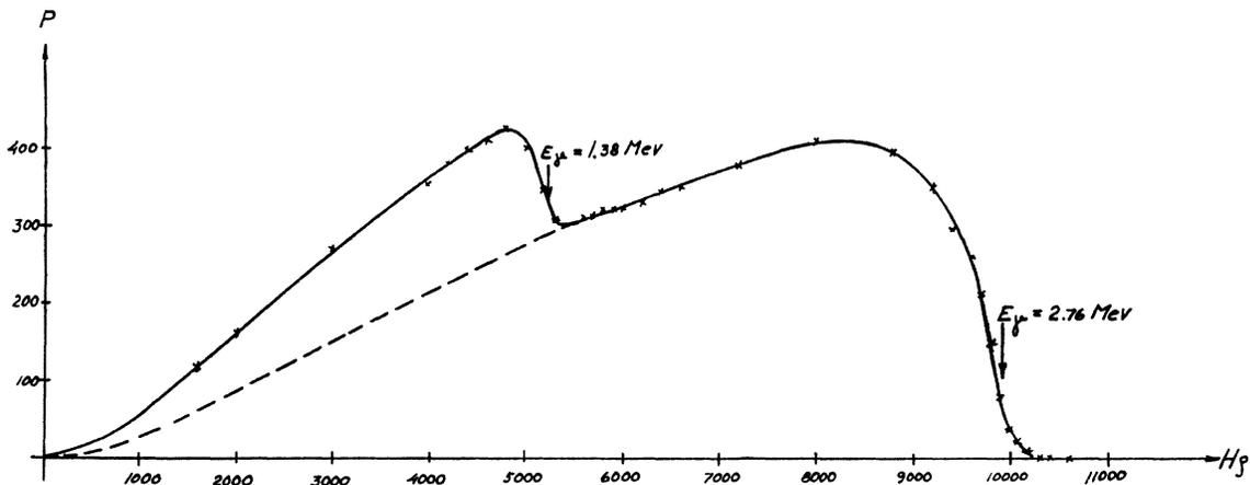
FIG. 2. Secondary electron spectrum expelled from a Cu radiator by the  $\gamma$ -rays of  $\text{Na}^{24}$ . The curve is in the undivided form.
