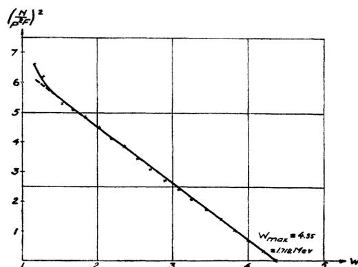
FIG. 7. The Fermi diagram for  $P^{32}$ .
