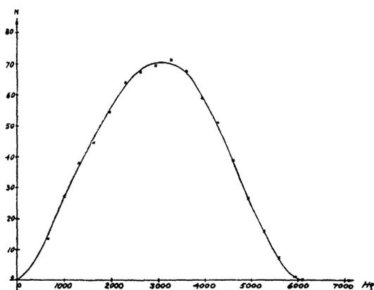
FIG. 4. The  $\beta$ -spectrum of  $\text{Na}^{24}$ .
