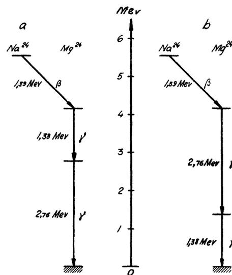
FIG. 8. Nuclear level scheme for the disintegration of  $\text{Na}^{24}$ .
