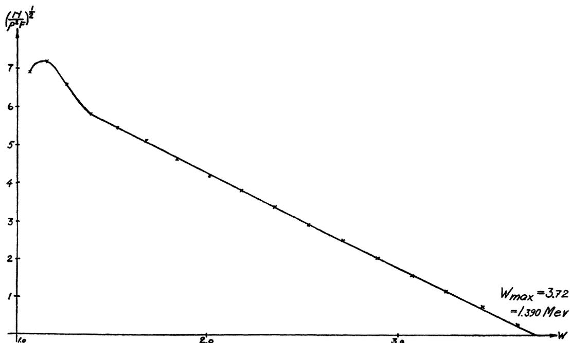
FIG. 5. The Fermi diagram for  $\text{Na}^{24}$ .
