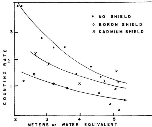
FIG. 1. Counting rate, in arbitrary units, observed with no shield and with boron shield, as a function of altitude.
