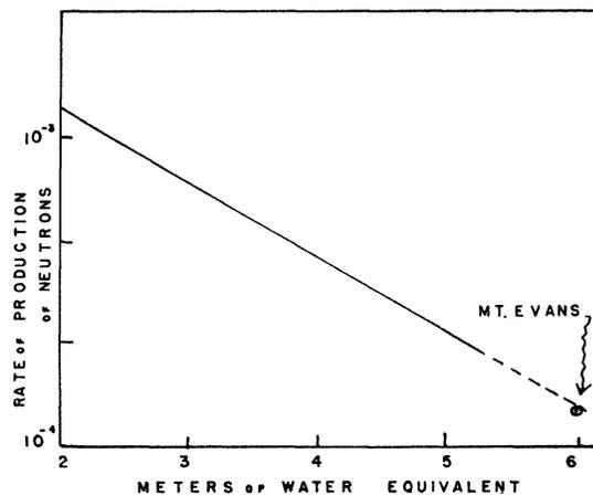
FIG. 2. Rate of production of neutrons by the cosmic radiation in the atmosphere;  $q$ , per gram per second, derived from Fig. 1, as a function of altitude. Point at 6 meters previously observed on Mt. Evans, for comparison.
