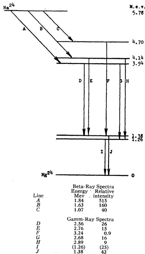
FIG. 4. Proposed term scheme for the nuclear transition  $\text{Na}^{24} \rightarrow \text{Mg}^{24}$ . Lines *I* and *J* have been observed as a single line by other investigators and no data on these lines are reported in this paper.
