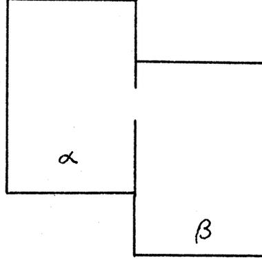
FIG. 7. Asymmetrical coupling of the two tuned cavities.
