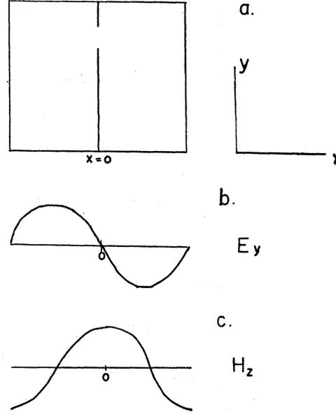
FIG. 4. Field distribution in the first mode  $\omega_1$  of two coupled tuned cavities. (a) Cross section of cavities. (b) Electric field  $E_y$ , as a function of  $x$  (same curve for any value of  $y$ ). (c) Magnetic field  $H_z$ .
