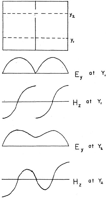
FIG. 5. Field distribution in the second mode  $\omega_2$  of the cavities of Fig. 4. (a) Cross section [identical with 4(a)]. (b) Electric field  $E_y$  along a line not going through the hole ( $y=y_1$ ). (c) Magnetic field along the same line. (d) Electric field  $E_y$  along a line  $y=y_2$  going through the hole. (e) Magnetic field along the same line.
