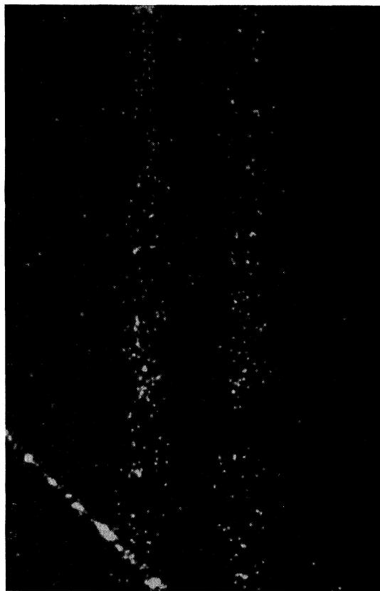
FIG. 1. An enlarged section of one of the mesotron tracks. The ions not only have diffused but also have separated into columns of plus and minus ions before the drops formed. The denser column of drops formed on the plus ions. The actual length of the portion of the original track here reproduced was 4 cm.
