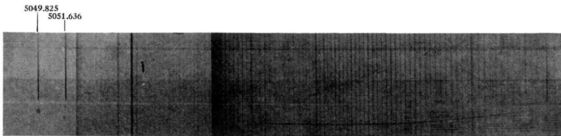
FIG. 2. An enlargement of the (0'-0) and (1-1) bands of the {}^1\Sigma \rightarrow {}^1\Sigma system at 5060 Å.
