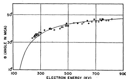
FIG. 7. The angle of progression of the radiation in mica as a function of the electron energy. The solid curve is the theoretical one obtained from Eq. (1). The open and closed circles represent experimental points obtained by two different samples of mica.
