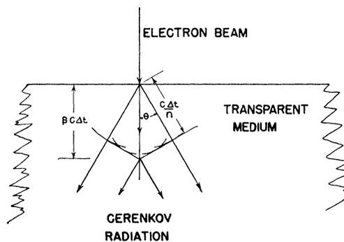
FIG. 1. Simple Huygens construction illustrating the formation of the wave fronts in the production of Cerenkov radiation. The electrons producing the radiation travel faster in the transparent medium than does the radiation which they generate. The radiation is symmetrical about the electron beam.
