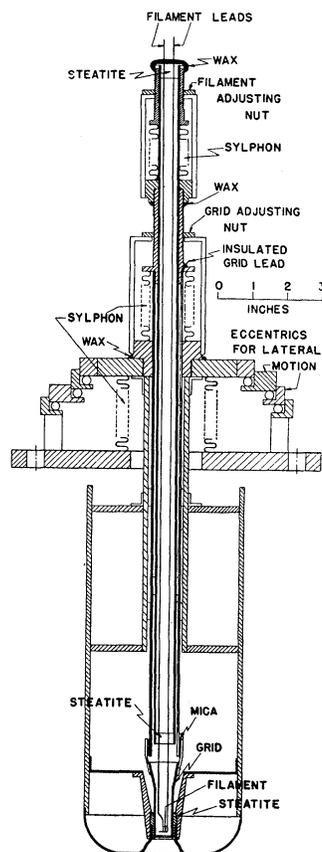
FIG. 3. The cathode assembly. The double eccentric permits a lateral adjustment of the whole cathode.
