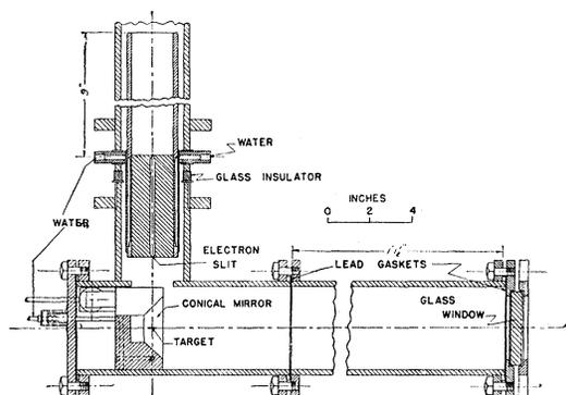
FIG. 4. The target and electron slit assembly. The electrons strike the mica target located on the axis of a  $45^\circ$  conical mirror. Radiation proceeding in a plane perpendicular to this axis is reflected parallel to the axis.
