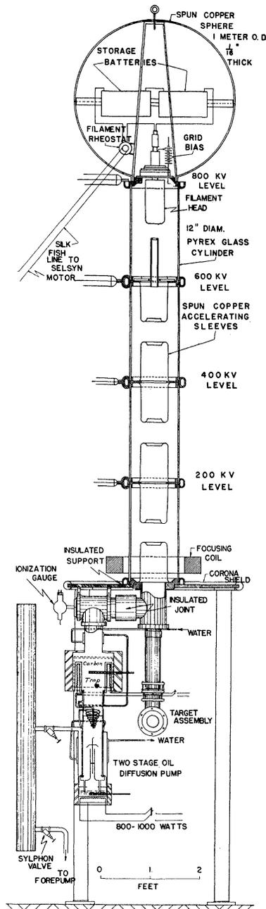
FIG. 2. A schematic diagram of the tube in which the high energy electrons are generated.
