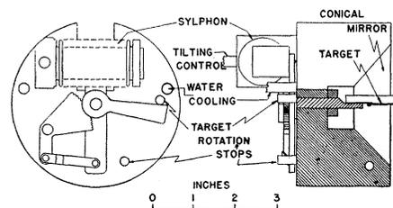
FIG. 5. Target tilting mechanism. The target must be tilted to avoid total reflection at the surface.
