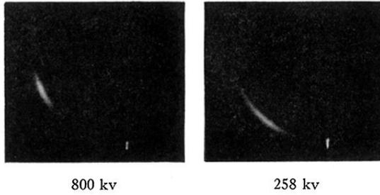
FIG. 6. Typical pictures of the radiation with the mica tilted  $20^\circ$  to the electron beam. After reflection from the conical mirror the radiation appears along the arc of a circle. The angle measured along the arc from the filament image at the bottom gives the angle of emergence of the radiation from the mica. The shift in angle of emission of the radiation with energy of the electron beam is readily visible.
