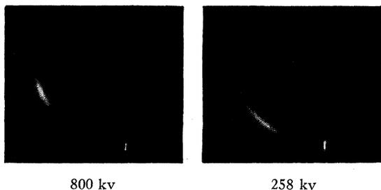
FIG. 6. Typical pictures of the radiation with the mica tilted  $20^\circ$  to the electron beam. After reflection from the conical mirror the radiation appears along the arc of a circle. The angle measured along the arc from the filament image at the bottom gives the angle of emergence of the radiation from the mica. The shift in angle of emission of the radiation with energy of the electron beam is readily visible.
