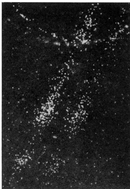
FIG. 1. Section of mesotron track 6949, enlarged to about three times its size in the cloud chamber. Ion pairs are separated into positive and negative columns, with the positive on the left side. At the top a sharp electron track crosses the picture.
