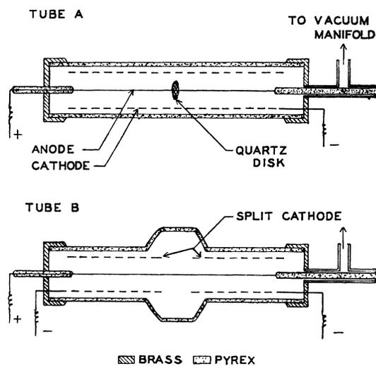
FIG. 1. Design of counters used to study discharge characteristics. Tube A, for study of localization phenomenon; Tube B, for study of effect of surface charge collected on walls of tube.
