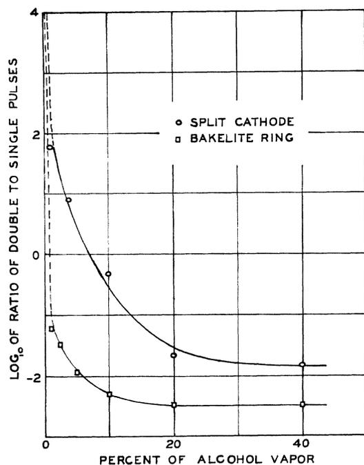
FIG. 2. Curves showing effectiveness of a Bakelite ring (No. 7, Table I) and a split cathode (No. 10) on localization of counter discharge for various mixtures of alcohol and argon.
