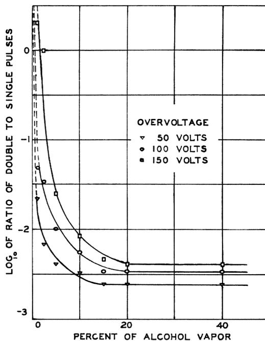
FIG. 3. Dependence of localization on the overvoltage at which the counter is operated.
