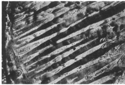
FIG. 4. Pattern on crystal A near grain boundary; normal applied field of 22 oersteds. Magnification 100 \times .
