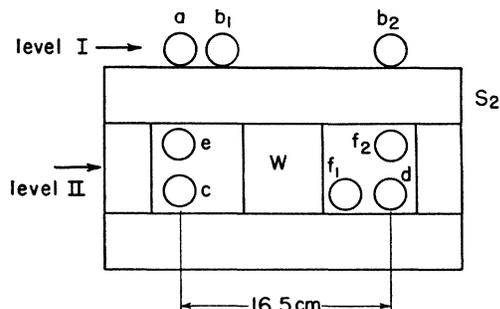
FIG. 3. Arrangement of counters for the detection of simultaneous penetrating particles.
