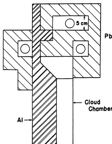
FIG. 5. Arrangement of cloud chamber and controlling counters, in vertical projection.
