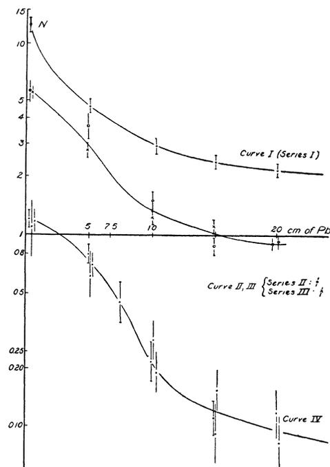
FIG. 2. Absorption curves for local air showers and for  $A$  showers.  $N$  is the number of coincidences per hour.
