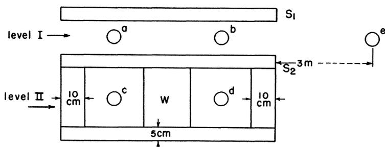
FIG. 1. Arrangement of counters and screens in the absorption measurements on local air showers and on  $A$  showers.
