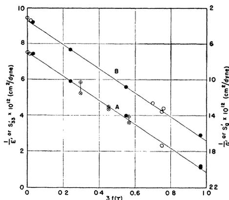
FIG. 1. Curve A, reciprocal of rigidity modulus; Curve B, reciprocal of Young's modulus, as functions of orientation. Lines and solid circles (●) are from Goens and Weerts. Other points are the writers' values. On Curve A, the symbols have the following significance: ○, no bending-torsion correction; ⊕, from "maximum slope" run; ⊗, from "minimum slope" run and correction factor  $\phi$ .
