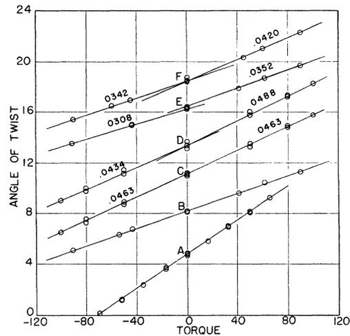
FIG. 2. Angle of twist against axial torque. Curve *A* is for a brass rod. Curves *B* to *F* are runs on lead single crystals. *B* and *C* are typical examples of straight line plots, while *E* and *F* are typical examples of runs of the double slope type. The slopes are shown by the numbers near the curves. The unit of torque is 1960 dyne cm and the unit of twist is  $5.6 \times 10^{-8}$  radian.
