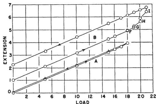
FIG. 4. Load against extension for crystal No. 1. Each unit of load produces a stress of  $0.415 \times 10^6$  dynes/ $\text{cm}^2$ . The zero load is  $0.67$  dyne/ $\text{cm}^2$ . Each unit of extension corresponds to a longitudinal strain of  $18 \times 10^{-6}$ . Curve B was taken directly after curve A and the ascending branch coincides with the descending branch of curve A, but is offset to avoid confusion. The first elastic limit observed for this crystal was at 14 on the load scale.
