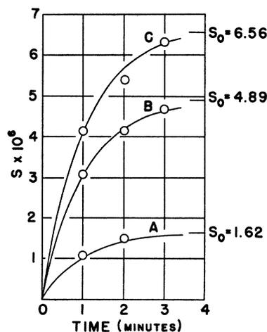
FIG. 5. Creep as function of time. Ordinate is longitudinal strain,  $S$ ; abscissa, time in minutes.
