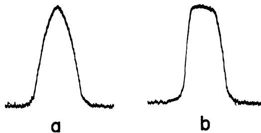
FIG. 8. Microphotograms of the electron beam spot: (a) in the horizontal plane, (b) in the vertical plane.
