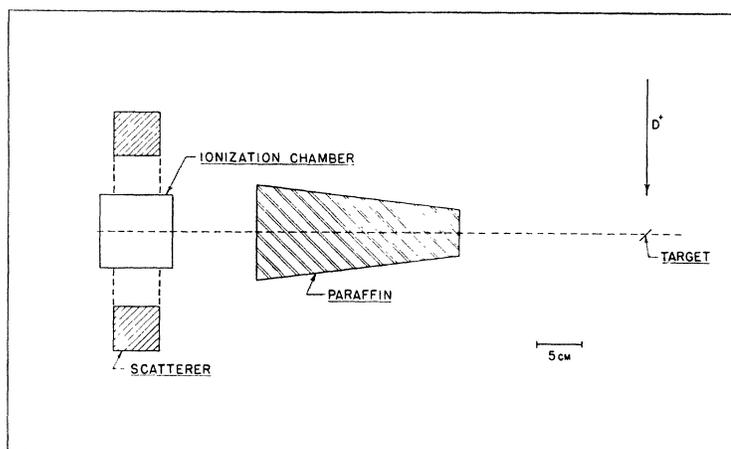
FIG. 1. Experimental arrangement for investigating the neutrons scattered through  $100^\circ$ .
