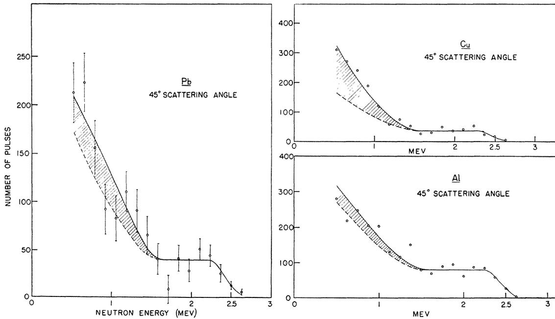
FIG. 4. Distribution in energy of recoiling  $\alpha$ -particles from neutrons which were scattered through  $45^\circ$  by Al, Cu, and Pb.
