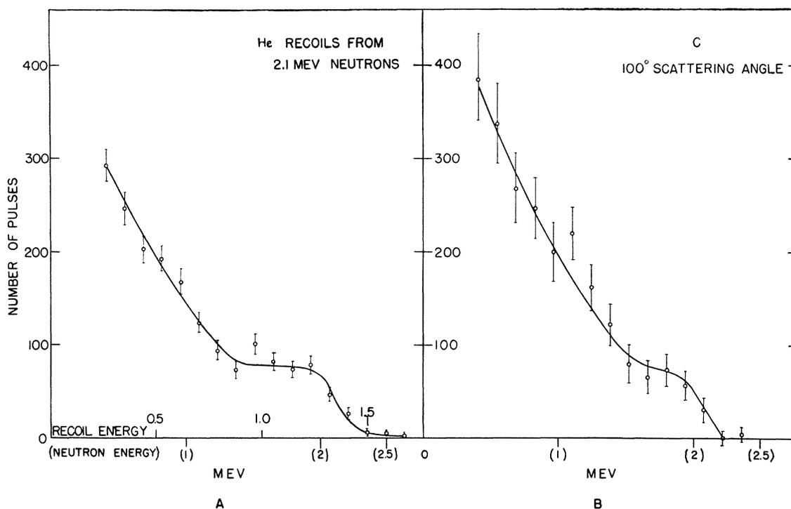
FIG. 6A. Distribution in energy of recoiling  $\alpha$ -particles knocked on by 2.1-Mev neutrons from the  $d-d$  reaction.
