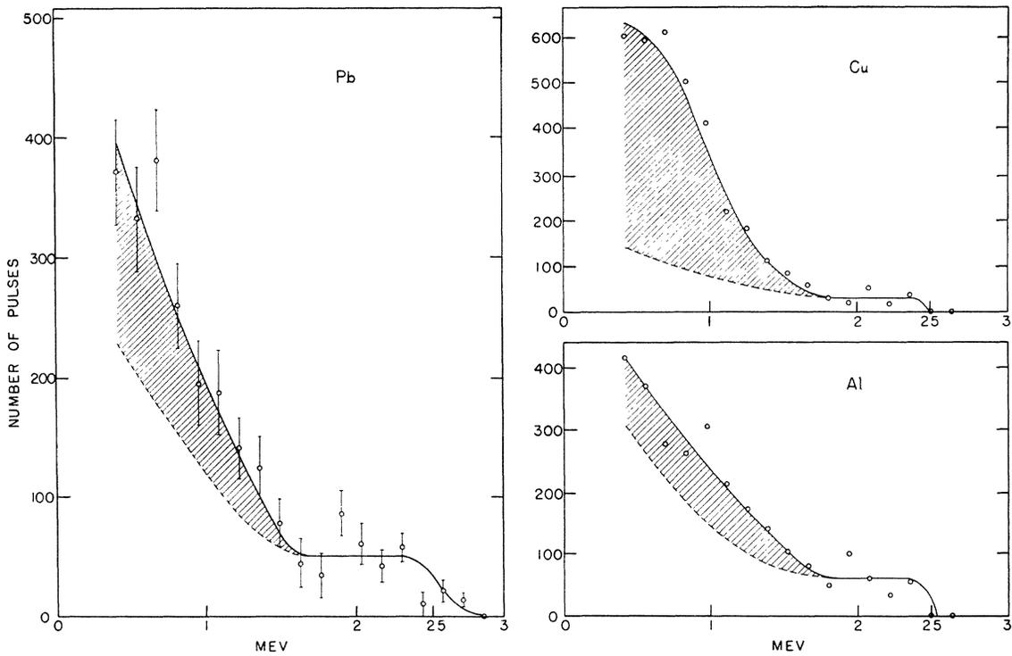
FIG. 3. Distribution in energy of recoiling  $\alpha$ -particles knocked on by neutrons which were scattered through  $100^\circ$  by Al, Cu, and Pb. The cross-hatched areas are a measure of inelastic scattering.
