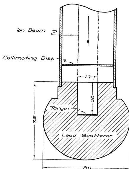
FIG. 1. Neutron source and scatterer. Dimensions are in cm. Cloud chamber 24 cm to right.
