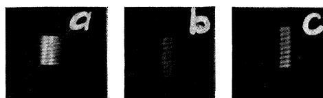
FIG. 2. Wide angle interference fluorescence of the salicylaldehyde compound of europium at 6100 Å. (a) \theta = 22.5^\circ , \chi/2 = 0^\circ ; (b) \theta = 45^\circ , unpolarized; (c) \theta = 45^\circ , \chi/2 = 90^\circ . \chi/2 = 90^\circ when the electric vector of the polarizing prism is perpendicular to the plane I, I' .
