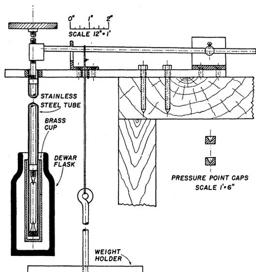
FIG. 1. The apparatus used for subjecting specimen cylinders to compressive stresses at various temperatures.
