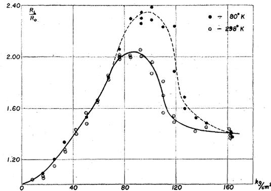
FIG. 2. The relative increase in internal friction as a function of compressive stress. The solid circles refer to data taken on specimens subjected to compression at  $80^\circ\text{K}$ . The open circles refer to data taken on specimens subjected to compression at  $298^\circ\text{K}$ .
