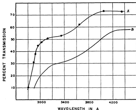
FIG. 8. Transmission of thin sample of crystal. Curve *A*—photo-cell. Curve *B*—photographic. Points on curve *B* were obtained generally at intervals of 10Å. No interval was larger than 25Å.
