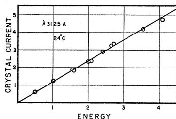
FIG. 4. Behavior of crystal current with respect to incident energy for constant voltage gradient.
