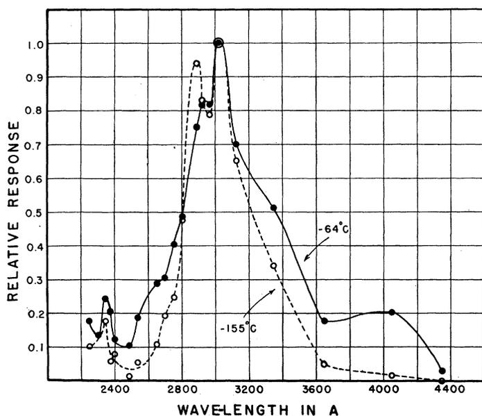
FIG 7. Photoconductivity at lower temperatures. See Fig. 6.
