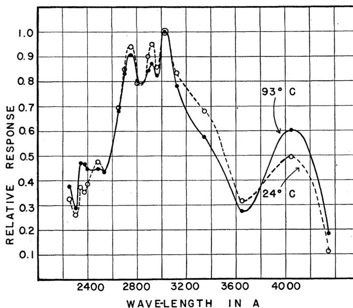
FIG. 6. Crystal current per unit incident energy (at constant voltage gradient) plotted against wave-length.
