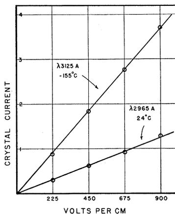
FIG. 5. Variation of crystal current (in arbitrary units) with voltage gradient at constant intensity of illumination.
