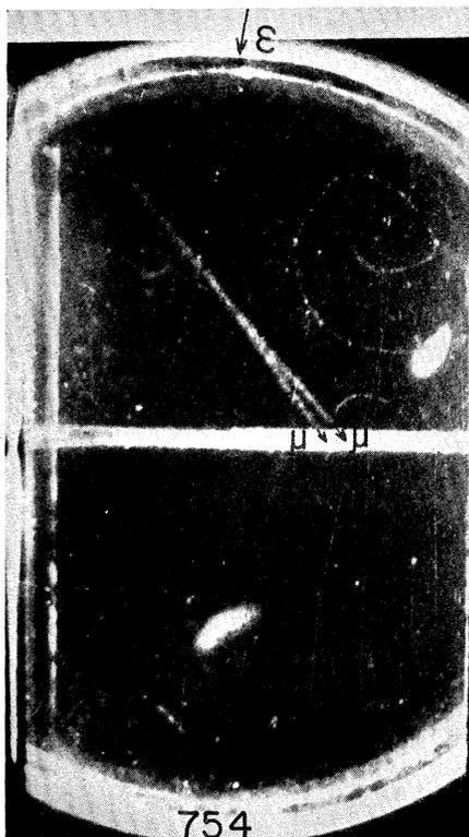
FIG. 3. Cloud-chamber photograph showing two particles stopped in 0.32 cm copper.
