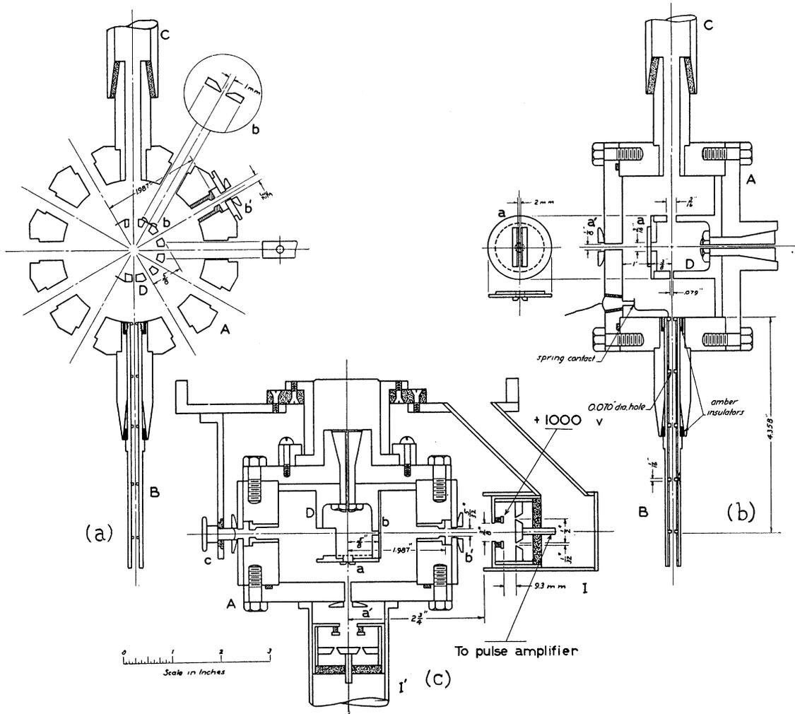
is allowed to escape from the target chamber before its main portion strikes a metal surface, in this case the bottom of an insulated cup *C*. This reduces the intensity in the vicinity of the ionization chambers of the neutrons produced where the beam is stopped, and thus aids in keeping down the background count.
