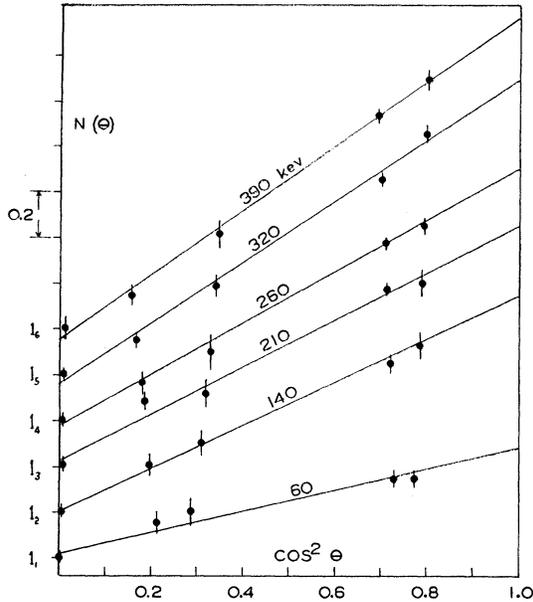
FIG. 3. Angular distribution of the ejected protons plotted against  $\cos^2 \theta$ . Note that the scale for successive curves is shifted 0.2 unit of ordinate. The length of the vertical bar through each point is equal to twice the statistical probable error of that point.
