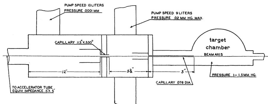
FIG. 1. Schematic diagram of pumping system used to maintain the necessary pressure differential between the target chamber and the accelerating tube.
