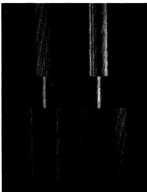
FIG. 1. Asymmetrical Zeeman patterns at 88,350 gauss produced by magnetic perturbations between terms y^5D_3^0 and y^5D_4^0 of Ru I. To the left, line 3100.839, to the right 3099.283A. The \pi components are above and the \sigma components below, while the center strip shows the two lines without magnetic resolution.
