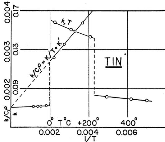
FIG. 4. Thermal conductivity of tin.  $k$  in cal. per sec. per cm per degree C.
