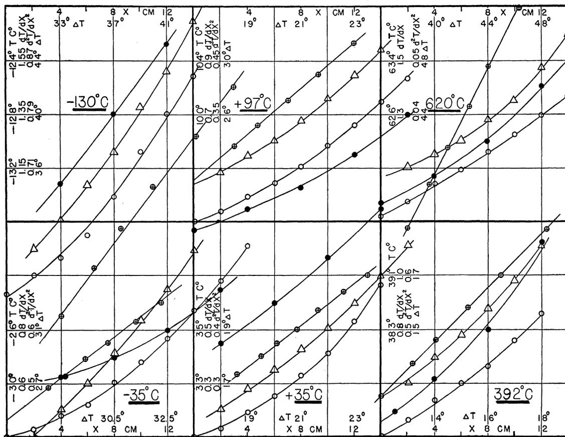
FIG. 1. Experimental data for lead at various temperatures.
