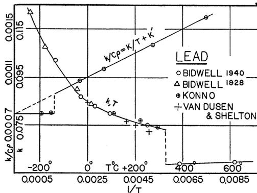
FIG. 2. Thermal conductivity of lead.  $k$  in cal. per sec. per cm per degree C.
