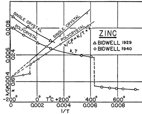
FIG. 3. Thermal conductivity of zinc.  $k$  in cal. per sec. per cm per degree C.
