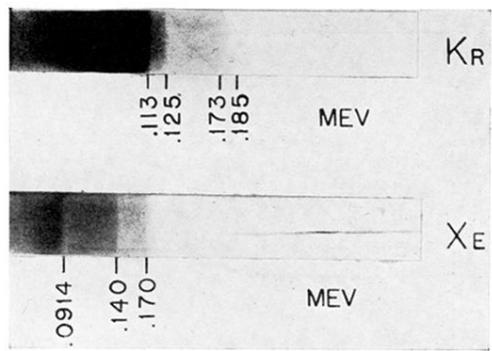
FIG. 3. Upper photograph: conversion electrons from krypton. Lower photograph: conversion electrons from xenon.
