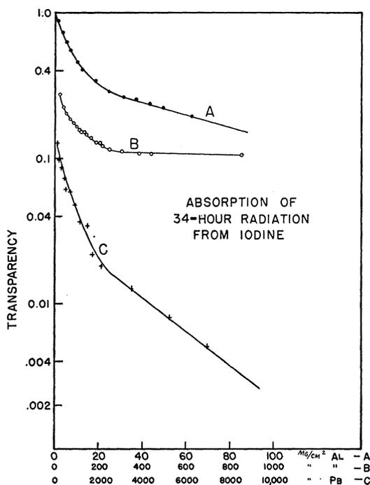
FIG. 8. Absorption of 34-day period from  $I^{127} + H^1$ . Curves A and B show absorption in aluminum. Curve C was made with lead absorbers but with 31 mg/cm<sup>2</sup> of aluminum between the absorber and the electroscop to remove the soft secondary radiation produced in the lead. Total activity was about 2 divisions/minute.
