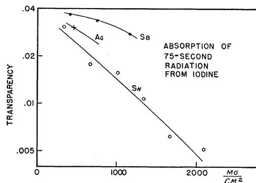
FIG. 6. Absorption of 75-second radiation from  $I^{127} + H^1$ , showing the x-rays are characteristic of xenon. Total activity was about 1 division/second. Absorption coefficients interpolated from data given in Compton and Allison, *X-Rays in Theory and Experiment*, are as follows: For iodine characteristic  $K$  radiation: in Sn,  $\mu/\rho = 9$ ; Ag, 62; Sb, 15. For xenon  $K$  radiation: in Sn, 45; Ag, 40; Sb, 10.
