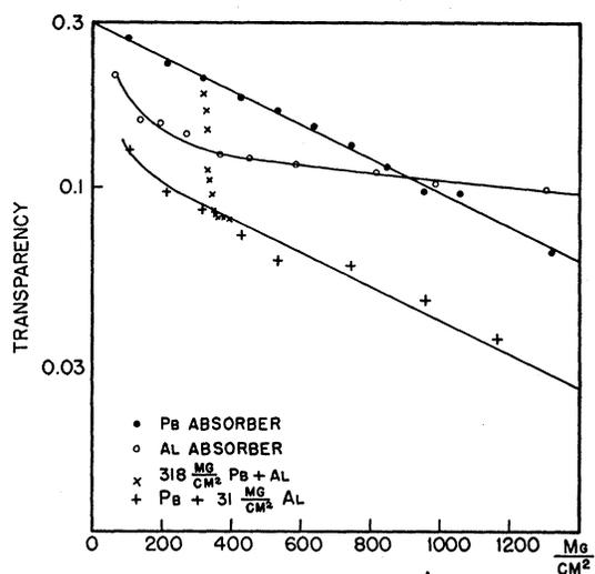
FIG. 9. Absorption of 34-day period from  $I^{127} + H^1$ . The filled-in circles show the absorption by lead alone; the open circles, by aluminum alone. The points marked  $\times$  were obtained by putting various thicknesses of aluminum between 318 mg/cm<sup>2</sup> of lead and the electroscop. The points marked  $+$  show the activity observed through lead absorbers, but with 31 mg/cm<sup>2</sup> of aluminum absorbing the secondary electrons produced in the lead.
