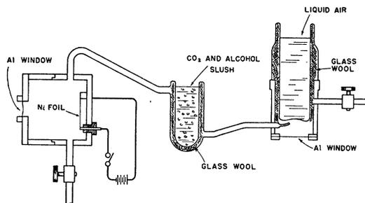
FIG. 2. Apparatus used to freeze out the radioactive krypton.
