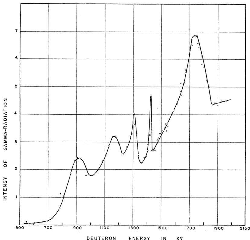
FIG. 1. The excitation curve for the emission of  $\gamma$ -rays from a thin target of carbon bombarded by deuterons. Open circles refer to data taken with an argon-filled ionization chamber and solid circles to data taken with coincidence Geiger counters.
