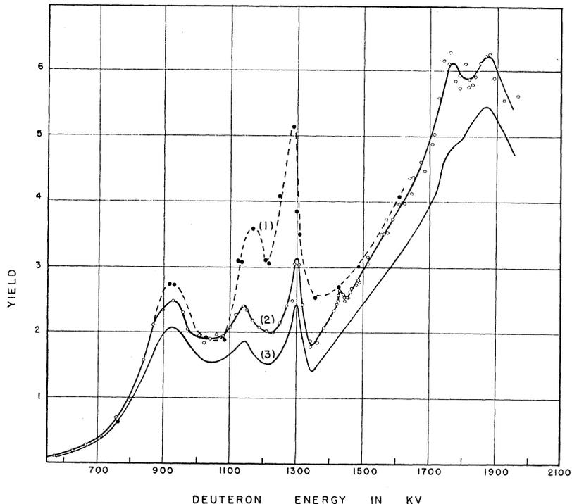
FIG. 1. Excitation curves for the emission of neutrons from a thin target of carbon bombarded by deuterons. Curve (1) gives the yield of  $N^{13}$  produced in the reaction. Curve (2) shows the ionization in a hydrogen-filled ionization chamber. Curve (3) is obtained from curve (2) by subtracting the effect produced by the  $\gamma$ -rays from carbon. Hence curve (3) represents the neutron yield.
