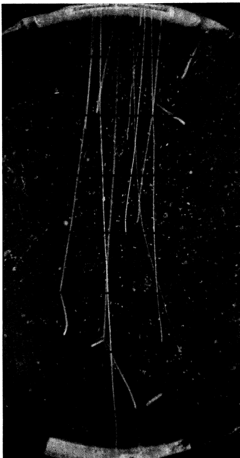
FIG. 1. Protons from aluminum bombarded by deuterons.
