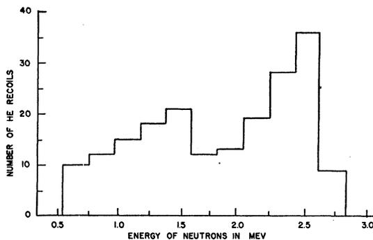
FIG. 2. Number of helium recoils observed as a function of the neutron energy producing the recoils.
