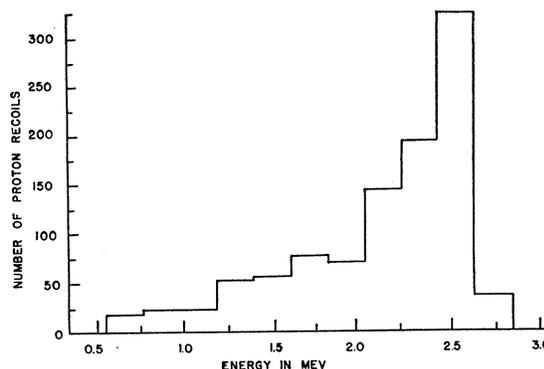
FIG. 3. Number-energy distribution of recoil protons produced in methane and in ethane.
