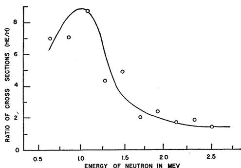
FIG. 4. Ratio of the backward scattering cross section for neutrons by helium and by hydrogen as a function of the neutron energy.
