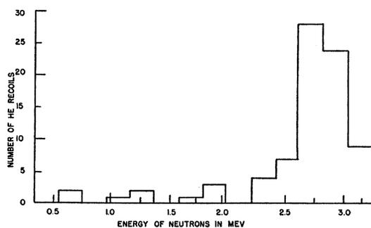
FIG. 6. The  $d-d$  neutron spectrum as observed in helium at  $51^\circ$ , under conditions identical with previous work by Baldinger, Huber and Staub.
