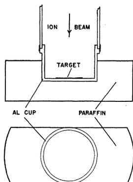
FIG. 1. Top and side views of the neutron source, showing the distribution of paraffin about the target. The cloud chamber was placed about 15 cm to the right.
