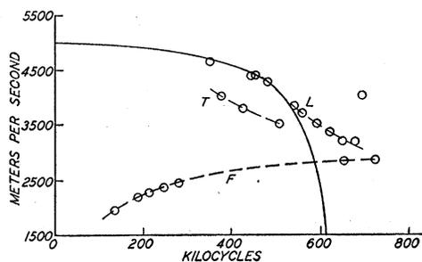
FIG. 6. Dispersion curves for the smaller nickel rod. Length: 25.45 cm. Mean diameter: 5.500 mm. *L*, *T*, and *F* denote the longitudinal, torsional, and flexural branches, respectively. The full line denotes the Giebe and Blechschmidt theoretical curve.
