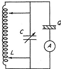
FIG. 1. Diagram of the crystal circuit.
