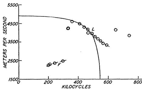
FIG. 3. Dispersion curves for the larger magnesium rod. Length: 14.98 cm. Mean diameter: 5.895 mm. *L* and *F* denote the longitudinal and flexural branches, respectively. The full line denotes the Giebe and Blechschmidt theoretical curve.
