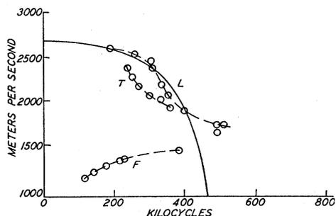
FIG. 5. Dispersion curves for the smaller silver rod. Length: 25.78 cm. Mean diameter: 4.057 mm. *L*, *T*, and *F* denote the longitudinal, torsional, and flexural branches, respectively. The full line denotes the Giebe and Blechschmidt theoretical curve.
