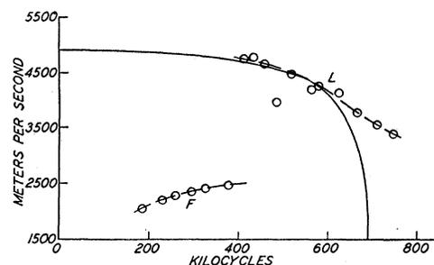
FIG. 4. Dispersion curves for the smaller magnesium rod. Length: 16.42 cm. Mean diameter: 4.615 mm. *L* and *F* denote the longitudinal and flexural branches, respectively. The full line denotes the Giebe and Blechschmidt theoretical curve.
