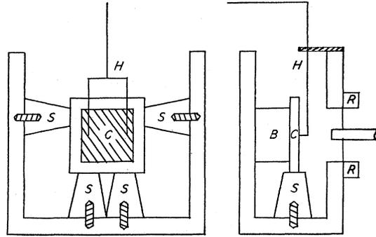
FIG. 2. Two sections of the crystal holder.  $S$ , stand-off insulators;  $H$ , high potential lead;  $C$ , quartz crystal;  $R$ , steel ring;  $B$ , brass cylinder.
