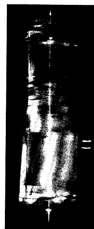
FIG. 3. Photograph of the projection tube in which was mounted the single crystal wire used for the measurement of the thermionic constants reported in this paper. The two white marks set off the portion of the crystal upon which the measurements were taken.
