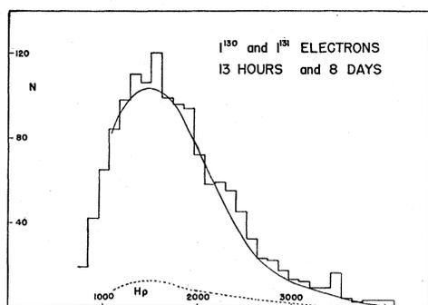
FIG. 8. Solid curve—momentum distribution of electrons from  $I^{130}$ . Broken curve—momentum distribution of electrons from  $I^{131}$ .
