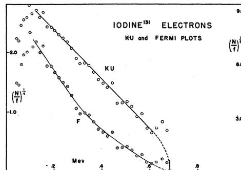
FIG. 7. Fermi and K-U treatments of I<sup>131</sup> electrons.
