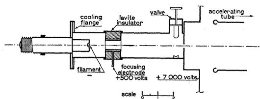
FIG. 2. The electron source.
