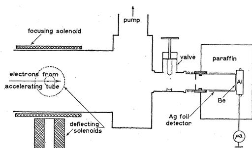
FIG. 3. Target arrangement.
