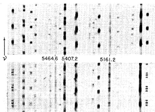
FIG. 1. Enlarged reproductions of spectrograms taken with 5.3 mm interferometer spacer showing  $\pi$  components in hyperfine Zeeman patterns of iodine; above at 4900 gauss, below at 9200 gauss.
