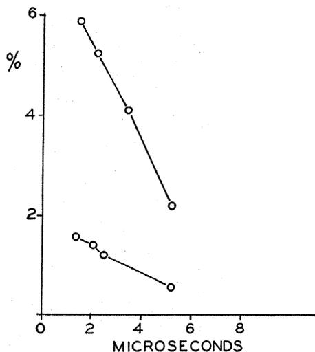
FIG. 5. The percentage of discharges of the counters (ordinate) which are delayed more than a certain time (abscissa) after the passage of the ray through the counter. Upper curve, 9 cm Hg pressure; lower curve, 18 cm Hg pressure.
