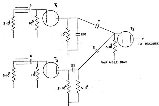
FIG. 2. Circuit for selecting the delayed coincidences.
