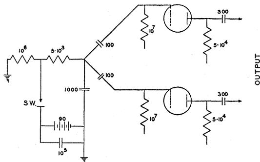
FIG. 3. Calibrating circuit for measuring the sensitive times of the coincidence selector circuit.
