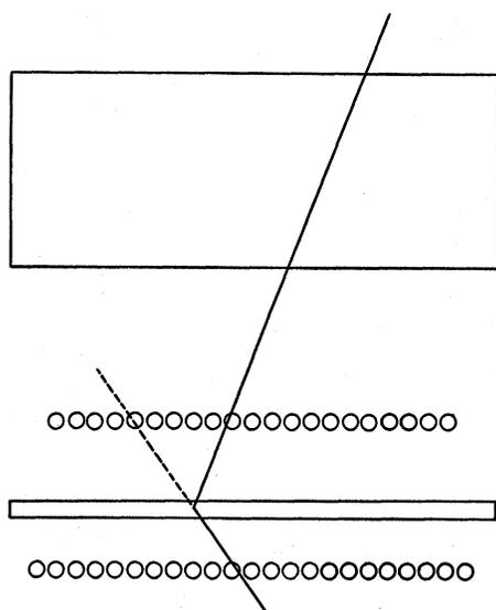
FIG. 1. Schematic diagram of the counter arrangement. A slow meson discharges one of the upper counters, stops in the thin lead plate, and some time later emits a neutrino and an electron which discharges one of the lower counters.
