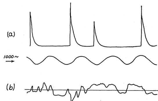
FIG. 5. Typical oscillograms of positive point streamer (A) and burst corona (B). In (B) the large d.c. component does not appear.
