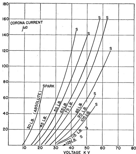
FIG. 4. Corona current *vs.* applied d.c. voltage for sulphur hexafluoride in a 3-mm point-to-plane gap, point positive.
