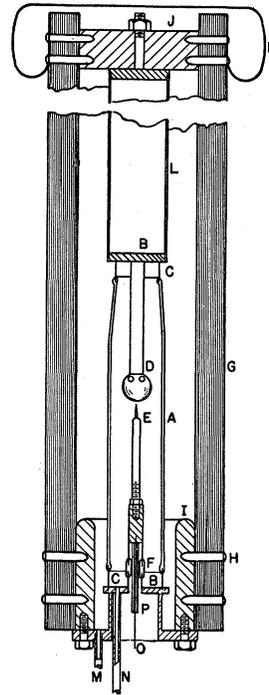
FIG. 1. Test cell installed in pressure jacket.
