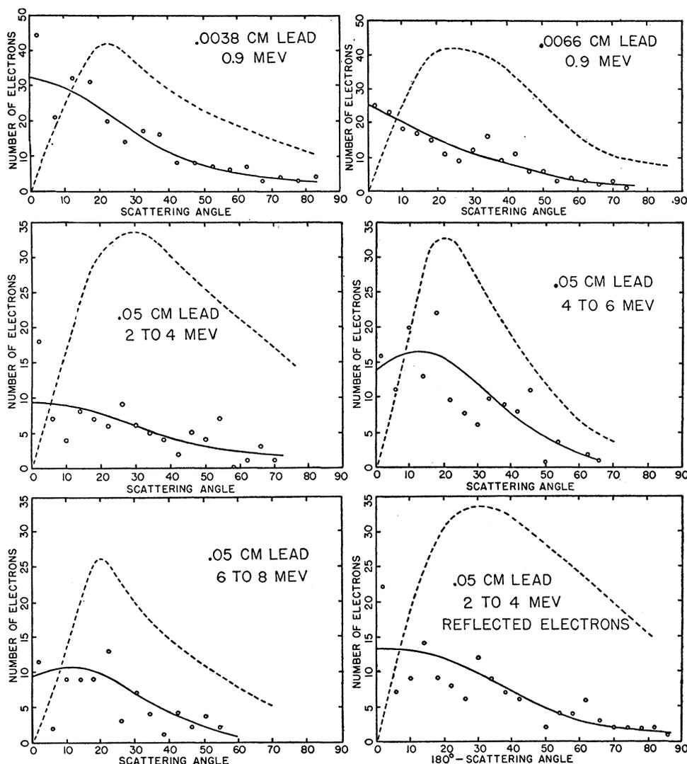
FIG. 3. Angular distribution of electrons scattered by lead.
