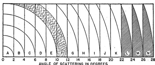
FIG. 1. Graphical device which is used in obtaining the true (three-dimensional) angular distribution of scattered electrons, from the cloud-chamber data.
