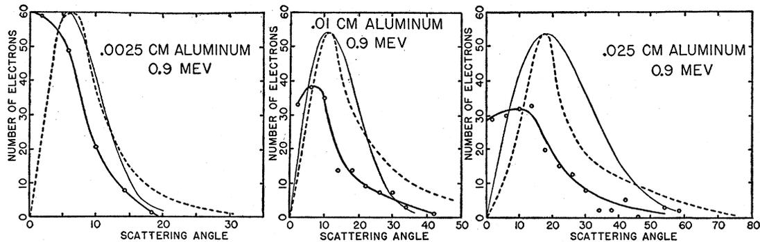
FIG. 2. Angular distribution of electrons scattered by aluminum.
