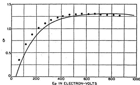
FIG. 1. Secondary yield vs. primary energy for nickel.
