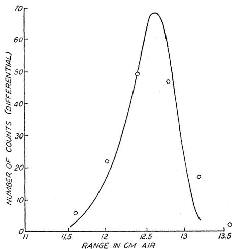
FIG. 5. Differential number-range curve for the  $\alpha$ -particles from  $\text{Li}^6 + \text{D}^2$ . The experimental points are from Fig. 4. The curve is calculated by taking into account penetration in the target and straggling.
