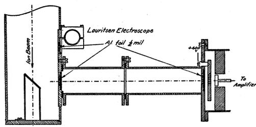
FIG. 2. Diagram of target tube, absorption tube, ionization chamber and monitor electroscop for measuring the number-range curve for the  $\alpha$ -particles from lithium bombarded with deuterons.
