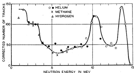
FIG. 1. Energy distribution of the neutrons from lithium bombarded with deuterons. The energy of the neutrons was measured by recoils in helium and hydrogen and the relative intensities corrected for geometry of the cloud chamber and scattering cross sections.
