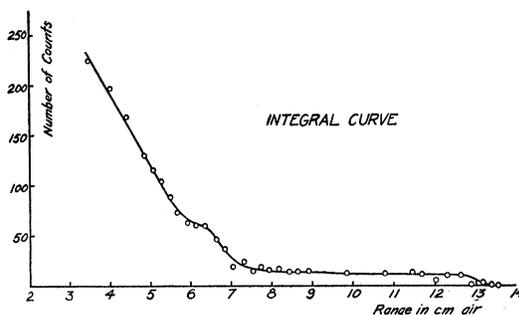
FIG. 3. Integral number-range curve of the  $\alpha$ -particles from lithium bombarded with deuterons.
