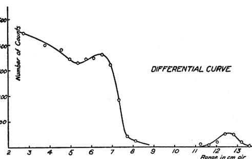
FIG. 4. Differential number-range curve of the  $\alpha$ -particles from lithium bombarded with deuterons.
