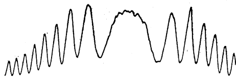
FIG. 1. Microphotometric record of the Be I line \lambda 4573A .
