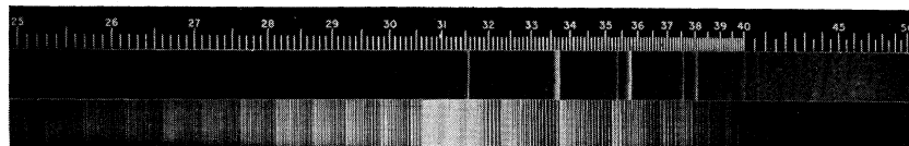
FIG. 4. Comparison of ozonizer and arc excitation in oxygen.
